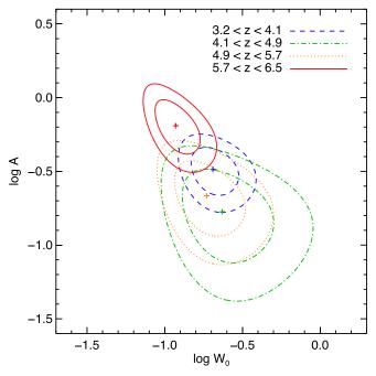
**Figure 3.** Results of the exponential fit to the distribution of O I  $\lambda$ 1302 equivalent widths for  $W_{1302} > 0.05$  Å. The contours show the 68% and 95% likelihood bounds over each redshift interval for the parameters in Equation (2); A is the number density of absorbers per unit path length integrated over all  $W_{1302}$ , and  $W_0$  is the exponential cutoff scale. Plus signs mark the highest-probability values.
