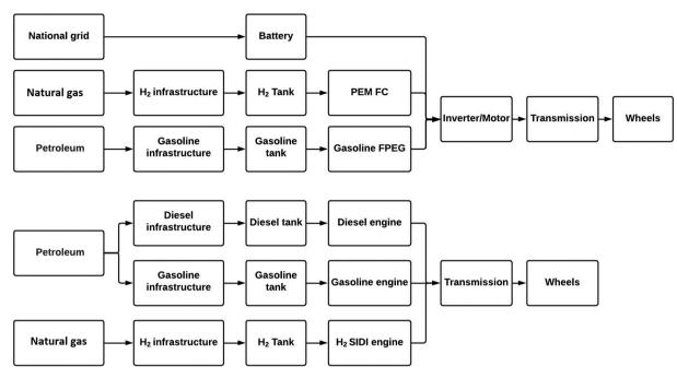
Fig. 5. Various powertrains technology layouts.
