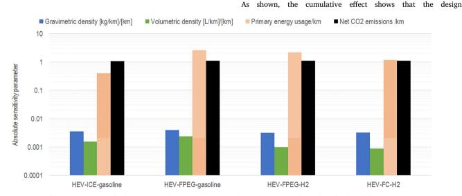
Fig. 11. Sensitivities of volume, mass, primary energy consumption and net CO<sub>2</sub> to the % electrification of the REEV.
