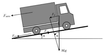
Fig. 2. Forces acting on the vehicle.
