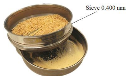
267 268 Fig. 4: Sieving of the fine fraction (smaller than 0.400 mm) of crushed soybeans.
