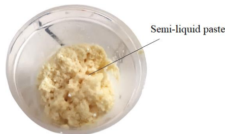
338 339 Fig. 9: Formation of a semi-liquid paste after addition of calcium chloride to test-tubes containing distilled water, 340 soybeans fine powder and urea (urea/calcium chloride concentration of 2.50 mol/L).
