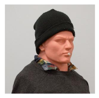
**Figure 2.** Picture of the manikin used to make binaural recordings. Anthropometric details of this manikin have been published elsewhere<sup>12</sup>. The center of the speaker used to generate emissions was placed at the mouth of the manikin (marked by a small tube).
