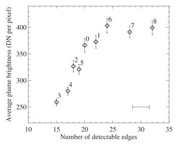
**Figure 10.** Average brightness of the plume (relative units) during the first nine time intervals (Intervals 0 through 8) shown in Figure 6, vs. the approximate number of plumelet edges identifiable in the Roberts-transformed images of the plume. Vertical error bars represent standard errors of average brightness measured in different longitudinal slices (see Figure 11); the horizontal error bar shows a typical uncertainty in counting the edges.
