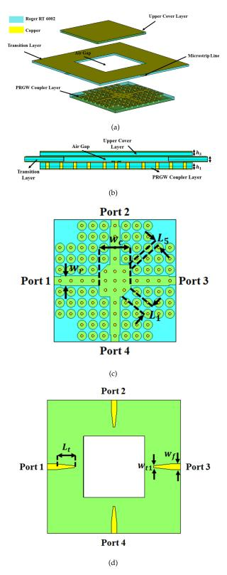
**FIGURE 3.** (a) 3-D geometrical configuration of proposed coupler. (b) Side-view. (c) Coupler layer. (d) Transition layer.
