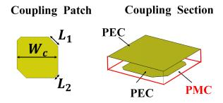
FIGURE 4. The proposed cavity resonator coupler model.
