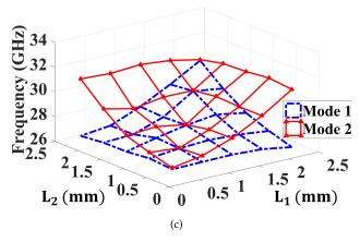
**FIGURE 5.** The effect of the cuts size on the resonance frequencies for different values of the coupling section width  $W_C$ . (a)  $W_C = 4.8$  mm. (b)  $W_C = 5$  mm. (c)  $W_C = 5.2$  mm.
