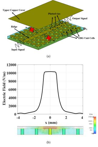
FIGURE 2. Wave propgation in PRGW structure. (a) PRGW line. (b) E-field distribution.
