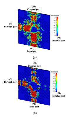
**FIGURE 6.** The E-field distribution of the proposed PRGW coupler at different frequencies. (a) F = 27 GHz. (b) F = 33 GHz.
