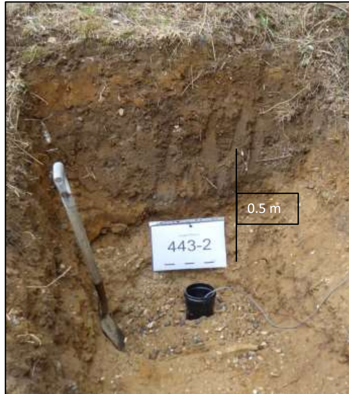
Figure SM1.3b Swanscombe Skull Site and Barnfield Pit, Kent, UK - trench cut into slope to access the Lower Gravel unit, showing back-filled sample location following sampling; in situ measurement in progress using a portable gamma spectrometer.
