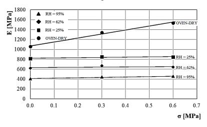
Figure 14: Stiffness envelopes of hyper-compacted earth mix 1 at different humidity levels.
