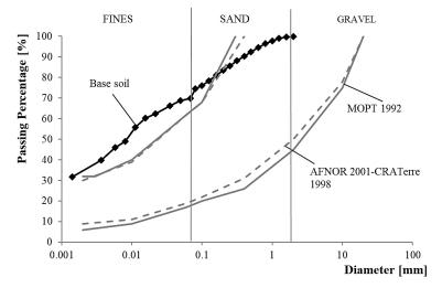
Figure 1: Particle size distribution of the base soil in relation to existing recommendations for the manufacture of compressed earth bricks by AFNOR [33]; CRATerre-EAG [34] and MOPT [35] (after Cuccurullo et al. [32]).
