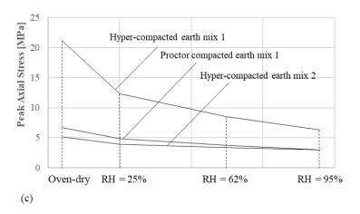
Figure 10: Evolution of peak axial stress as function of relative humidity at different confining pressures: unconfined (a), 300 kPa (b) and 600 kPa (c).
