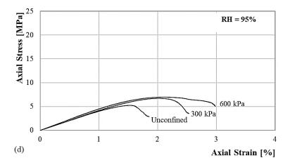
Figure 7: Results from triaxial tests on the hyper-compacted earth mix 1 at different confining pressures and distinct humidity levels: oven-dry (a), 25 % (b), 62 % (c), 95 % (d).
