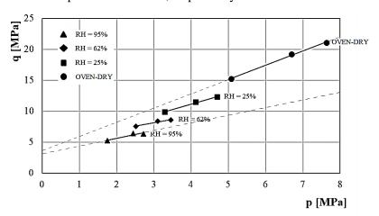
Figure 11: Strength envelopes of hyper-compacted earth mix 1 at different humidity levels.
