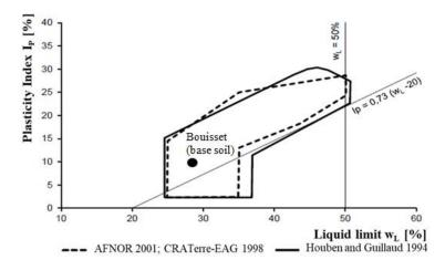
Figure 2: Plasticity properties of the base soil in relation to existing recommendations for the manufacture of compressed earth bricks by AFNOR [33]; CRATerre-EAG [34] and Houben and Guillaud [37] (from Cuccurullo et al. [38]).
