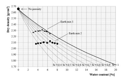
Figure 6: Hyper-compaction curves, corresponding to the application of a static pressure of 100 MPa, for earth mixes 1 and 2 (after Cuccurullo et al. [32]).
