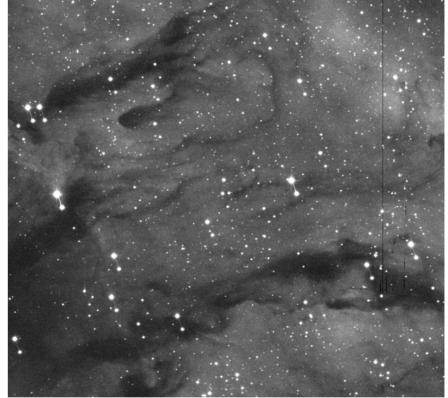
Fig. A.10. Double images on frame r367586, CCD#4. Bright stars clearly show the sign of INT mirror support oscillation, forming dumbbell-like images.
