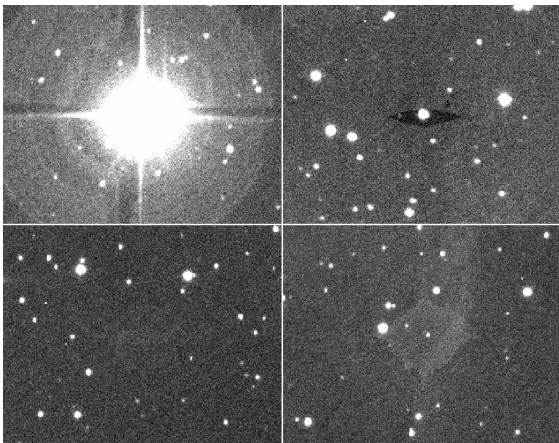
Fig. A.9. Cross talk on image r1023036: CCD#1 is shown top left, #2 top right, #3 bottom left, and #4 bottom right. The same pixel section is shown for each CCD. The bright star on CCD#1 is seen as a negative imprint on #2 for pixels that are saturated, as a positive imprint on #4, and as a faint positive imprint on #3.
