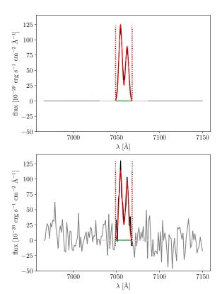
**Fig. A.3.** Noise-free (top) and noisy (bottom) template matches to the mock spectrum shown in Figure A.1. The top panel of Figure A.1 shows the same as the bottom panel of this figure. The red curve shows the FELIS template match to the part of the spectrum in black (within the vertical dotted lines). The green curve shows the template match before applying the flux scaling. The part of the mock spectrum outside the considered wavelength range is marked in gray.
