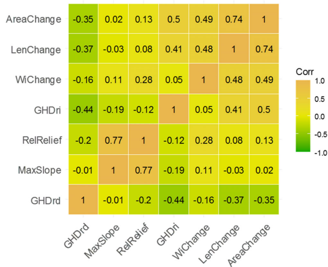
FIGURE 3 Correlation matrix for gully drivers. There are inverse associations between nearness to roads and changes in gully sizes. GHDri, gully head distance from rivers; GHDrd, gully head distance from roads; RelRelief, relative relief; WiChange, width change; LenChange, length change; Corr, correlation legend [Color figure can be viewed at wileyonlinelibrary.com ]
