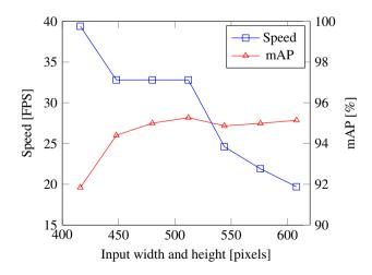
Fig. 6 Measurements of speed and mAP for detections performed by the axle detection network at varying resolution
