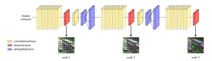
Fig.1 A simplified diagram of the YOLOv3 detection network, example detections and network layers are displayed for illustration purposes only and not shown to scale
