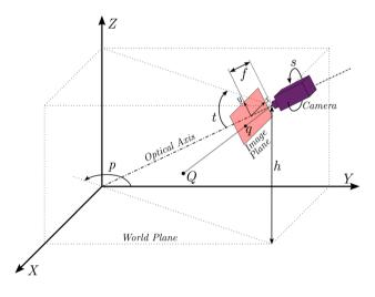
Fig. 2 General camera model (Based on [7])
