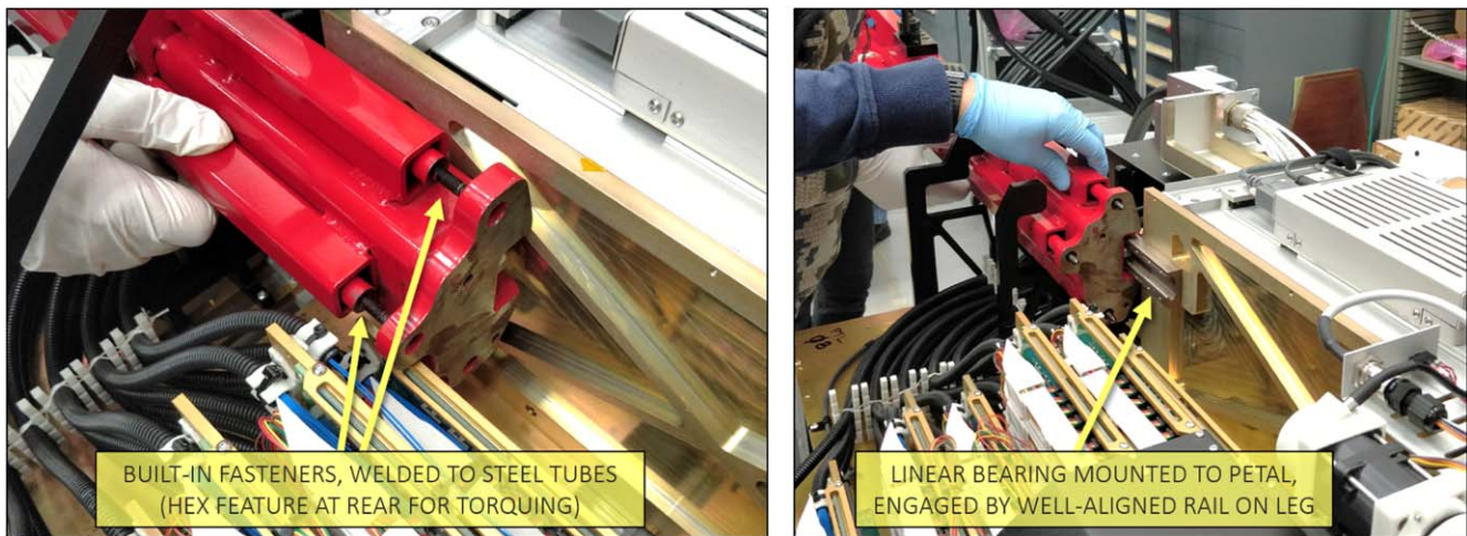
Figure 35. Petals are handled with a steel lift leg, with attachment points for horizontal (crane) and cantilevered (insertion fixture) attachment.
