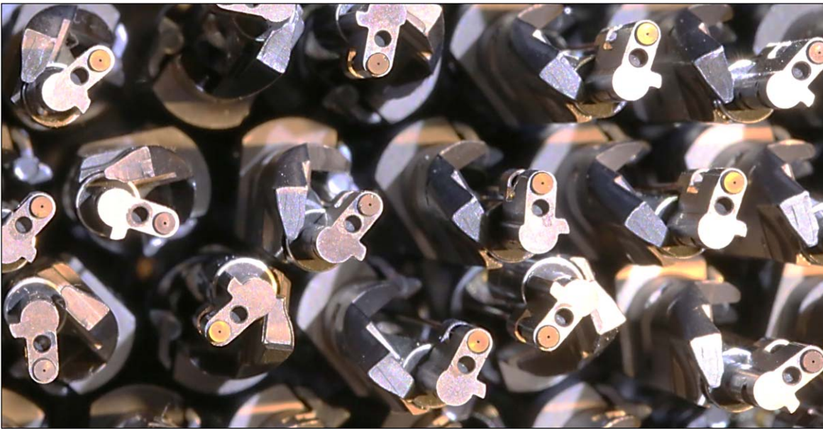
Figure 6. Fiber positioner robots are shown packed together on the focal plate. In addition to the fiber ferrule, each \phi arm has a light-trap hole with a dark dye. The original concept for these light traps was to be able to selectively extinguish bright stars in the field; in practice, they have been most useful for identifying \phi angles during hardware debugging. A projecting tab feature on each ferrule holder provides a simple but effective hard limit against clockwise overextension.
