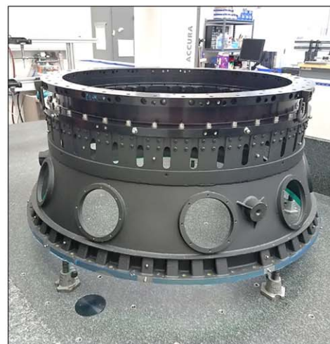
Figure 14. Left: key components of the focal plate structure include the steel FPD and aluminum FPD Ring, FPR, and petals. The FPD Ring is permanently bolted to the FPD via 40 flexural tabs, which accommodate the differential thermal expansion between the dissimilar metals of the Corrector Barrel and the Focal Plate. Right: FPD and FPR during alignment on a coordinate measuring machine.
