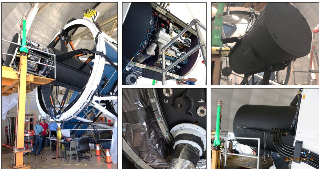
Figure 20. The thermal enclosure, shown with side panels off (left and center) and on (right). The heat exchanger can be seen in the upper center photo, surrounded by white MERV filter holders. The duct just below the heat exchanger wraps around the focal plane, injecting diffuse air flows at several ports into the volume between the C4 lens and the robots. At the lower center, the flexible air skirt is visible, adjacent to an air duct feeding into the FPD (the support structure that surrounds the volume between the C4 lens and the robot array).
