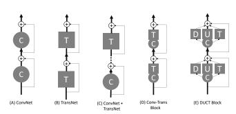
Fig. 1. Fig. 1. Comparison of existing convolution (A) and transformer (B) architecture designs with the proposed DUCT blocks. While previous work integrates convolution and transformer layers in a separate series (C), recent trends alternate transformer and convolution in a block-wise way (D). Our DUCT (E) is the proposed parallel structure combining a dynamic local enhancement module, a unary co-occurrence excitation module, and multi-head self-attention in a block-wise design.
