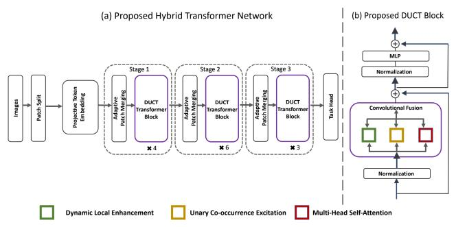
Fig. 3. (a) Architecture overview of the proposed hybrid transformer network DUCT. (b) The proposed hybrid transformer block for DUCT.
