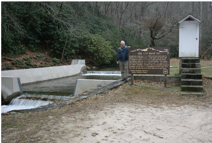
Fig. 9. The Coweeta Hydrologic Laboratory was one of several USDA Forest Service watersheds where the study of fluvial processes was much encouraged. This is the place where John Hewlett's influential work on hillslope hydrology was carried out. The photograph shows the main outflow from the Coweeta Basin: an unusual type of sharp-crested weir – a Cipoletti – is used to measure stream discharge. Standing by the weir is Wayne T. Swank, one of Coweeta's most important scientists. Source: T.P. Burt.
