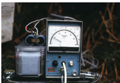
Fig. 7. The start of electronic field data collection in the mid-1970s: a conductivity meter linked to an electric chart recorder powered by a 12 V car battery. Source: photograph by T.P. Burt.
