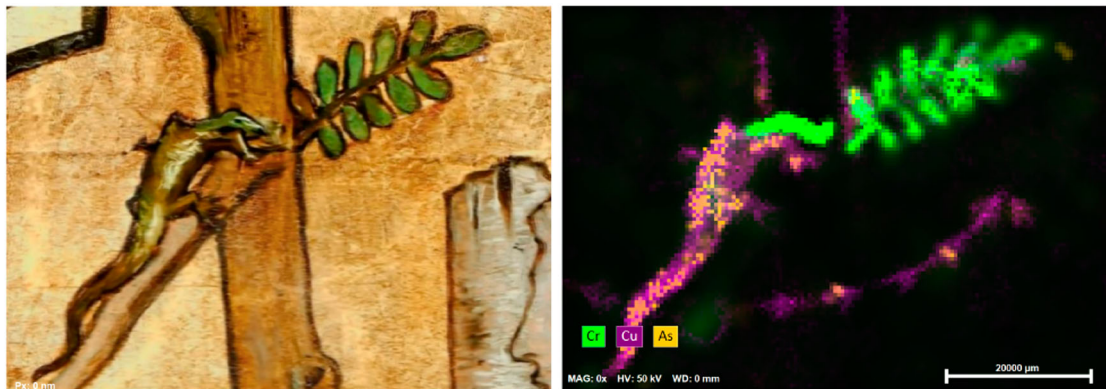
Figure 11. Visible images and false colour XRF map of chromium (green), copper (purple), and arsenic (yellow) on an area from the panel The origin of painting .
