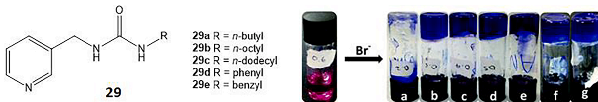
Fig. 34. Picture of the \text{Co}^{2+} - 29c metallogel in nitrobenzene and colour changed triggered by the addition of TBABr [(a) 0.2, (b) 0.3, (c) 0.4, (d) 0.5, (e) 1, (f) 2, (g) 4 equivs.]. Copyright RSC 2017. Reproduced with permission from ref [87].
