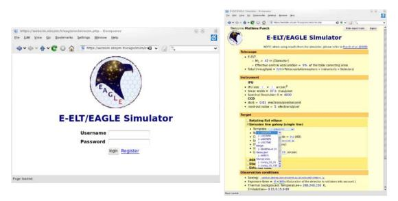
**Fig. 2.** Web pages of the EAGLE simulator. The user can pick up a science case using a menu (sed right-hand panel) and modify the parameters corrsponding to the telescope, instrument, object, sky, and detector, as listed.
