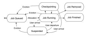
Figure 3: Job state transition diagram.
