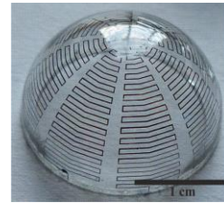
Fig.2 Electrically-small antenna on hemispherical substrate manufactured using holographic photolithography [14].
