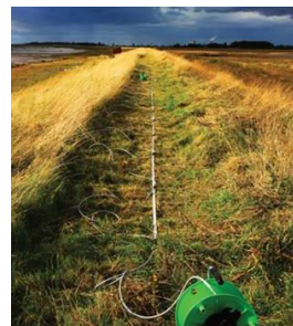
Figure 3. ERT monitoring along the crest of a flood embankment
