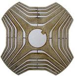
Fig.13. Rotor lamination.
