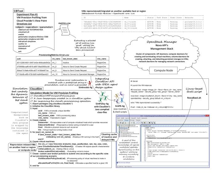
Figure 6: Execution of Scenario-1 to reprovision inactive/delayed VMs on another host
