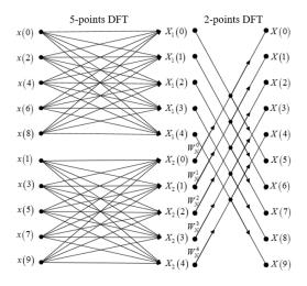
Fig. 3. Radix-2 and Radix-5 Mixed FFT structure
