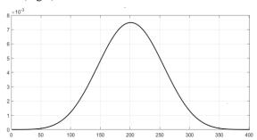
Fig. 2. weight window function  $\Psi$  (L=5,N=80)
