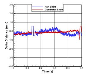
Fig.12. Flexible coupling, axially misaligned, ensemble average data
