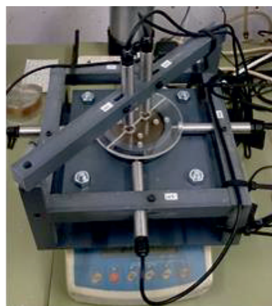
Figure 5. The laboratory set up for SWRC determination applying continuous hydraulic path changes (with tensiometer attached at the bottom).
