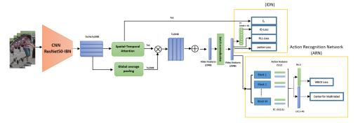
Figure 1: The proposed architecture with shared backbone (ResNet-50-IBN-a [30] and spatial-temporal attention [9]) followed by the IDN and ARN sub-network branches. ( $\otimes$  indicates pairwise multiplication;  $\oplus$  indicates summation).
