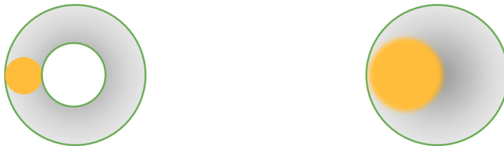
Figure 3. A phase screen (grey) positioned at (left) the pupil (orange) with screen #1 Ø83mm and (right) at a finite altitude (meta-pupil) with screen #2 Ø92mm. The largest pupil size of Ø24mm is illustrated with the altitude of screen #2 at the maximum position.
