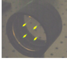
Figure 5. A previous example of a fluorescent cell being illuminated by 532 nm and having a peak re-emission wavelength of \approx 580 nm. The illuminating laser reflection can be seen on the entrance and exit windows with the fluorescence occurring in between, where the dye is in solution, and so can be separated via a dichoric.
