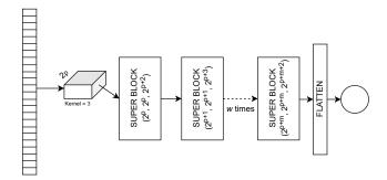
Figure 6: The ultimate design of our ResNet model
