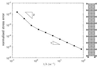
Figure 4. Column compression stress error
