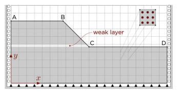
Figure 5. Slope geometry & boundary conditions
