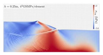
Figure 7. Deformed slope shaded by  $\sigma_{xy}$  for the ghoststabilised GIMPM
