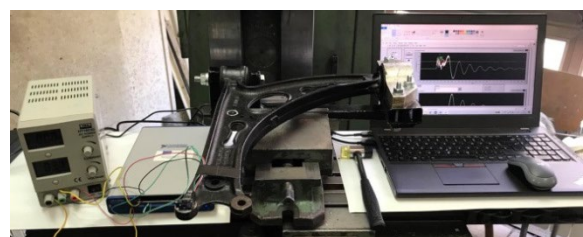
Fig. 7. Experimental determination of natural frequencies.
