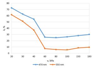
Fig. 10. Dependence of the contrast k of the mark on the frequency v, kHz for a sample of carbon steel C 75.
