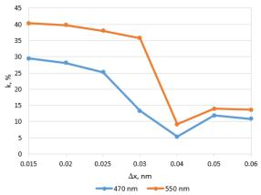
Fig. 9. Dependence of the contrast k of the mark on the step  $\Delta x$  for a sample of carbon steel C 75.
