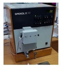
Fig. 6. Single-beam spectrophotometer with microprocessor "SPEKOL 11".
