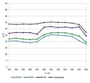
Fig. 8. Dependence of the reflection coefficient as a function of the wavelength for marked samples for the second experimental series.
