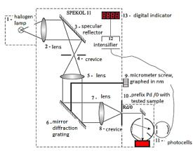
Fig. 5. Scheme of spectral reflection coefficient measurements with SPEKOL 11 spectrophotometer and attachment Rd/0.
