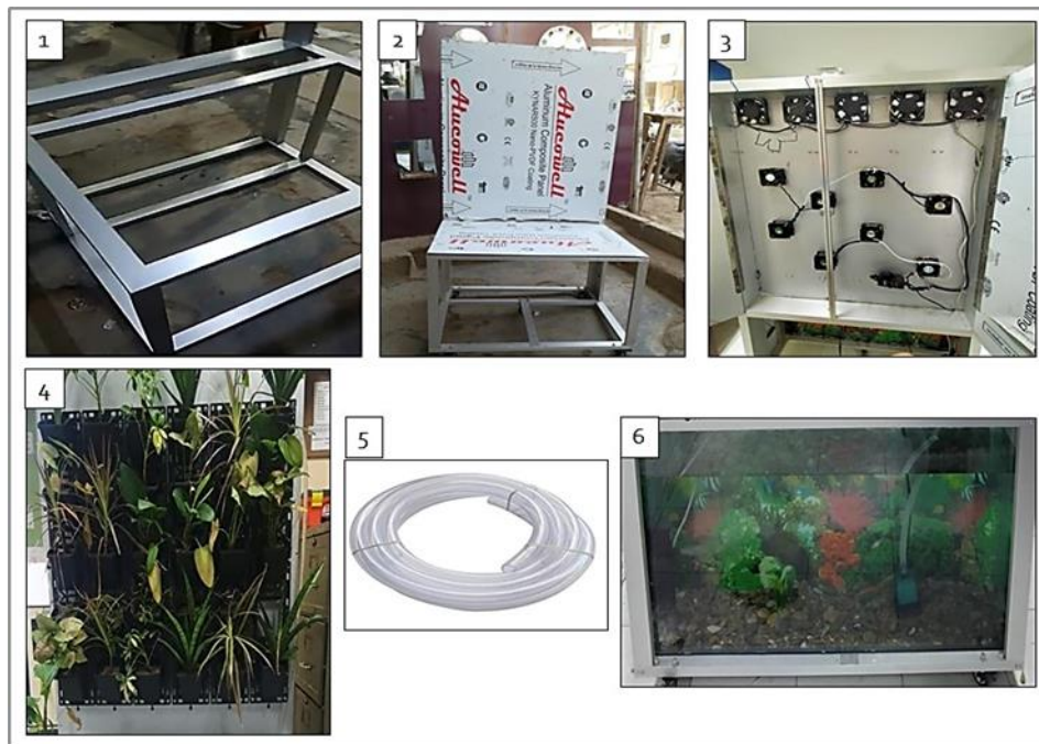
Figure 1. Fabrication phase (1) Bottom structure frame (2) Top cover of aluca bond sheet (3) Back view of fans placement at the top and center (4) Pots and plants (5) Irrigation pipe and (6) Aquarium and pump
