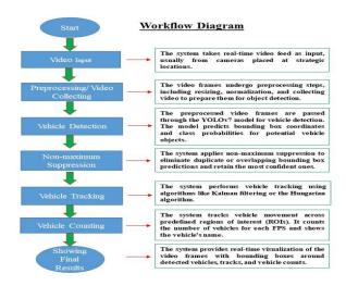
Fig. 2. Workflow diagram of system.
