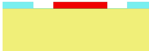
Figure 3.9: The cross-section of a CPW resonator. The yellow part is the substrate. The blue part is the ground. The red part is the center pin.
