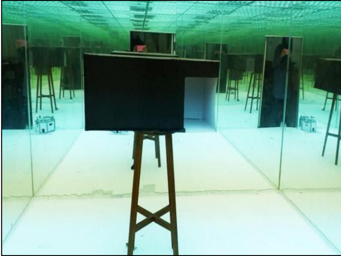
Figure 7: Scale Model Under Artificial Sky
