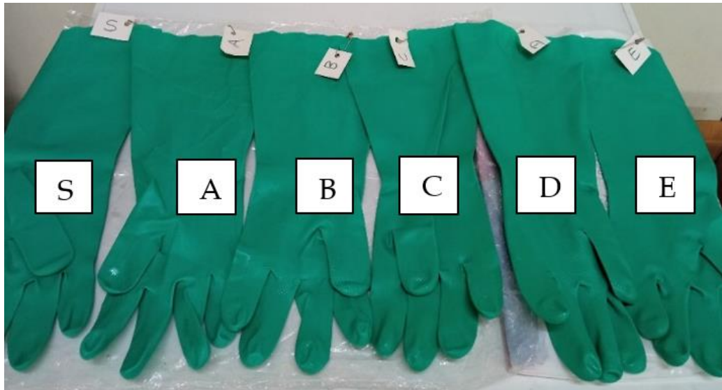
Figure 1. NBR latex glove samples; (S) control and HS treated (A) once in 15 min, (B) once in 30 min, (C) once in 1 hour, (D) once in 2 hours (E) once in 3 hours
