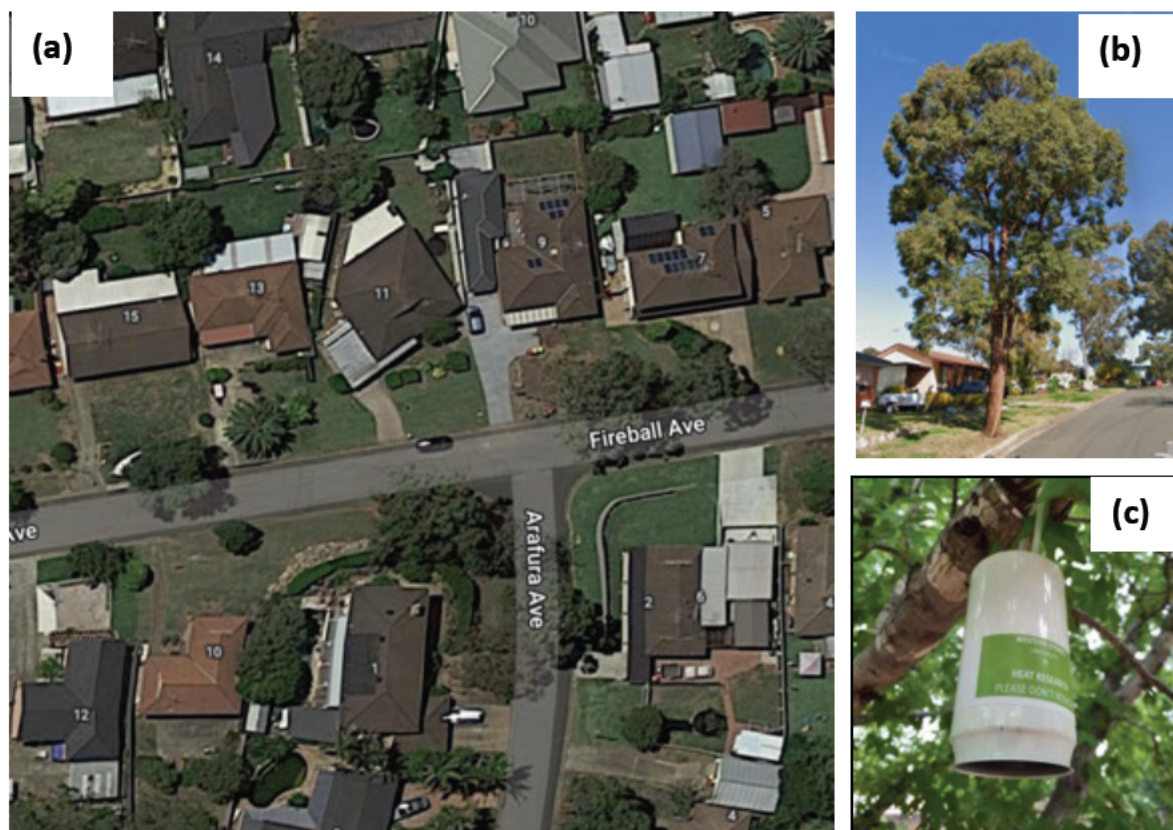
Figure 3. 1 (a) Example of the urban morphology of the studied suburb, Cranebrook, (b) trees ( Eucalyptus microcorys located on Arafura Avenue, Cranebrook), and (c) sensor and shielding affixed to a tree. The street map of Cranebrook shows that trees are growing on nature strips (verges) and at varying distances from houses. Images of (a) and (b) were sourced from google maps.
