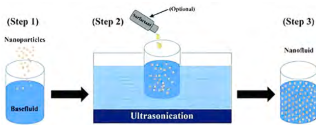
Fig. 2. Two-step liquid state nano-refrigerant preparation technique [26].
