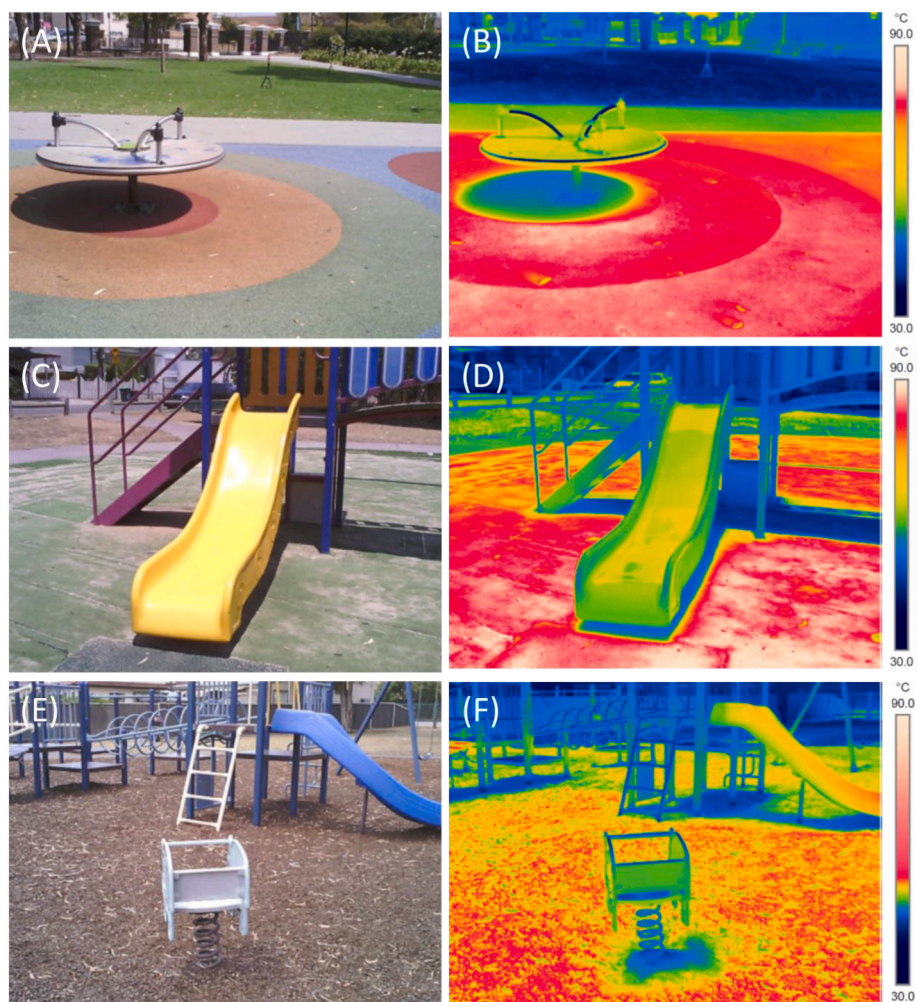
Fig. 1. [2-column fit]. Normal red-green-blue (A, C, E) and infrared (B, D, F) images of in-situ playground surface temperatures at 3 of the 10 playgrounds visited within metropolitan Sydney (NSW, Australia). Images were taken at Auburn Park at 15:30 h (A, B), Bunnalong Park at 13:30 h (C, D), and Colquhoun Park at 14:20 h (E, F) on 4 January 2020. Colour scales on the right-hand side indicate the range of surface temperatures ( ^{\circ}\text{C} ) measured.
