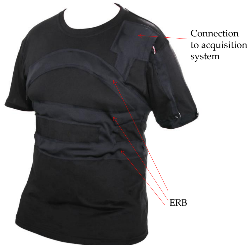
Figure 2. Third-generation ERB morphic sensors fully assembled in a t-shirt (image courtesy of Medical Monitoring Solutions Pty Ltd., Sydney, Australia).
