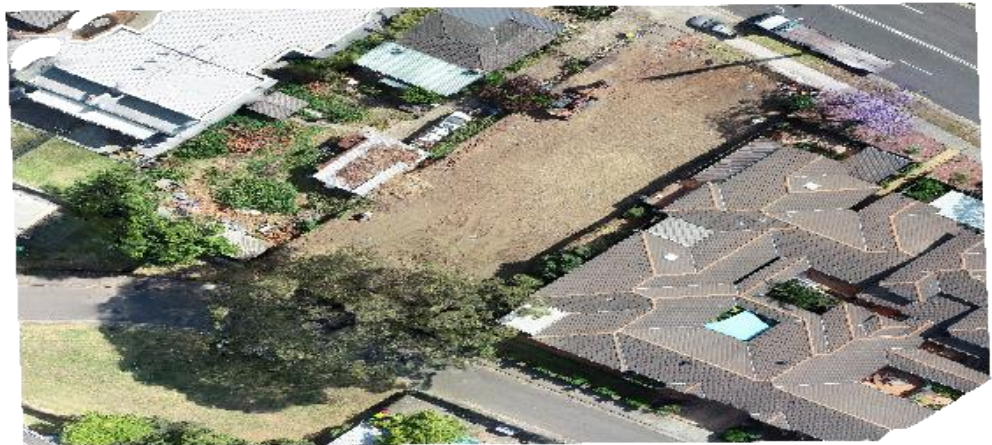
Figure 5. 3D orthomosaic map for the case study, generated from series of photos taken by the UAS and processed via photogrammetric software (Pix4D Platform).
