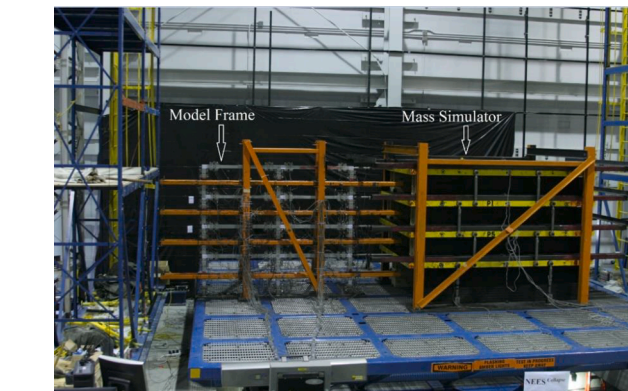
Fig. 4. Test structure, mass simulator, and bracing system on the SUNY-NEES shake table [82].
