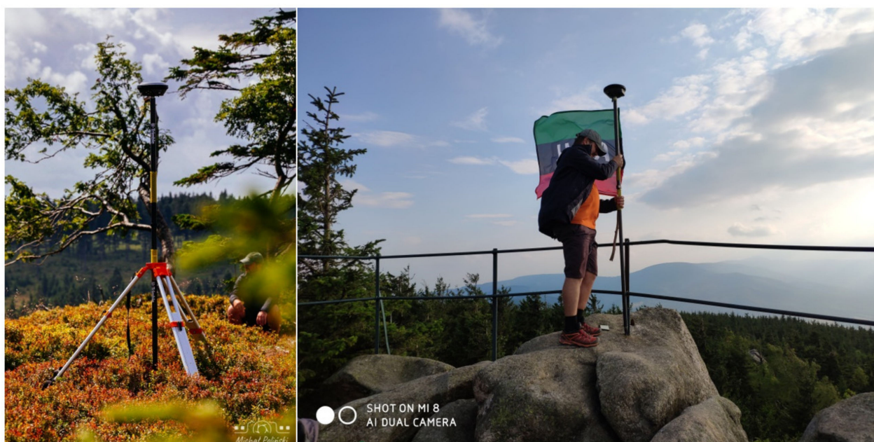
Figure 5. GNSS static session at Mount Brusek (the Złote Mountains, on the left) and RTK measurement at Mount Ostra Mała (the Rudawy Janowickie Mountains, on the right). Author: Krystian Kozioł.
