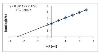
Figure 4. Potentiometric method (standard addition method) for electrode (ENR+DBPH+PTA) at concentration 10<sup>-3</sup> M of ENR drug.
