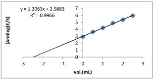
Figure 5. Potentiometric method (standard addition method) for electrode (ENR+DBPH+PTA)at concentration 10<sup>-4</sup> M of ENR drug.
