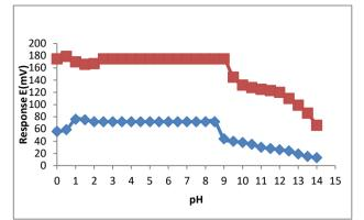
Figure 3. Values of pH for (ENR+DBPH+PTA) and (ENR+DOP+PTA) sensors at 10<sup>-3</sup> M of drug.
