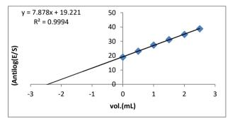
Figure 6. Potentiometric method (standard addition method) for electrode (ENR+DBPH+PTA) at concentration 10<sup>-3</sup> M of ENR tablets.
