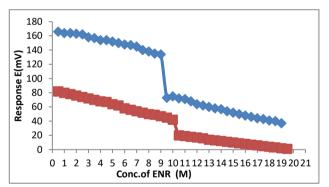
Figure 8. Potentiometric method (titration method) for electrode (ENR+DBPH+PTA)at concentration 10<sup>-3</sup> M of ENR drug and PTA.
