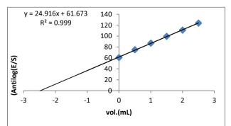
Figure 7. Potentiometric method (standard addition method) for electrode (ENR+DBPH+PTA) at concentration 10<sup>-4</sup> M of ENR tablets.
