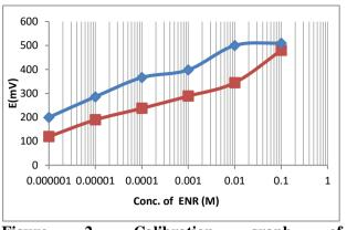
Figure 2. Calibration graph of (ENR+DBPH+PTA) and (ENR+DOP+PTA) electrodes.
