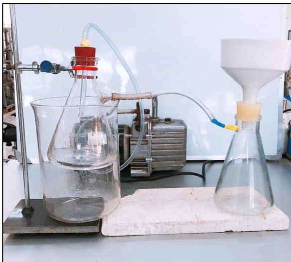
Figure 2. Photo of the filtration unit.
