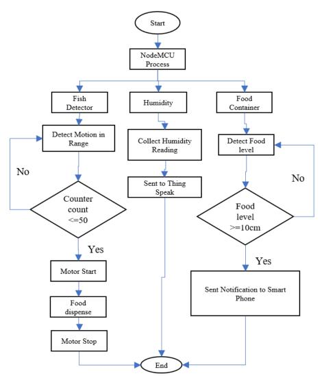
Figure 1. Flowchart of Automatic Fish Feeder
