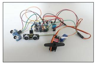
Figure 5. The hardware design of Auto Fish Feeder
