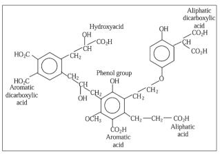
Figure 1. Hypothetical molecular structure of humic acid, showing important functional groups<sup>6</sup>
