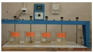
Figure 3. Jar test used for the experiments
