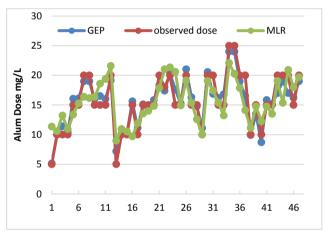
Figure 13. Comparing the observed data with the results of the two models
