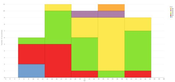
Figure 10. Optimal alum dose frequency for each initial turbidity used at the four sets of experiments
