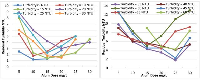
Figure 6. Residual turbidity for different alum dose and different initial turbidity
