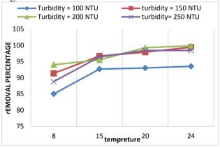
Figure 15. Turbidity removal at different temperatures for high turbidity concentrations
