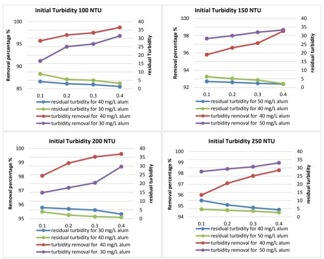
Figure 16. Residual Turbidity when using different starch doses as coagulant aid
