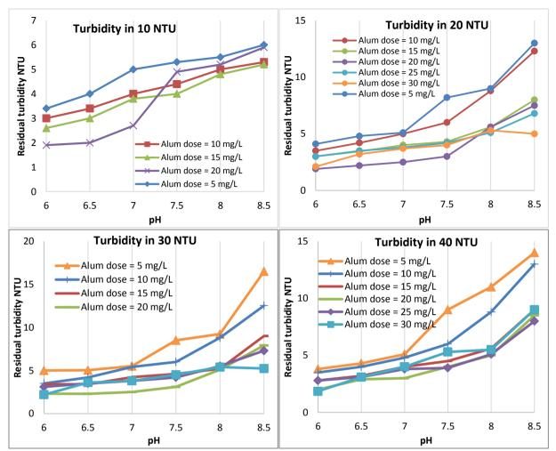
Figure 7. Residual turbidity for different pH level at different initial turbidity
