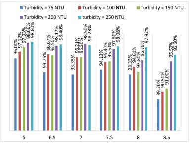
Figure 14. Turbidity removal for different pH levels at high turbidity concentrations
