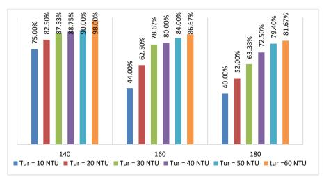
Figure 9. Turbidity removing percentage for different alkalinity levels
