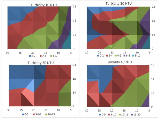
Figure 8. Residual turbidity for different alum dose at different temperatures
