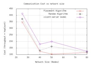
Figure 5. Communication Cost against different network sizes.
