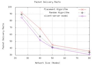
Figure 7. Packet Delivery Raito against different network sizes.
