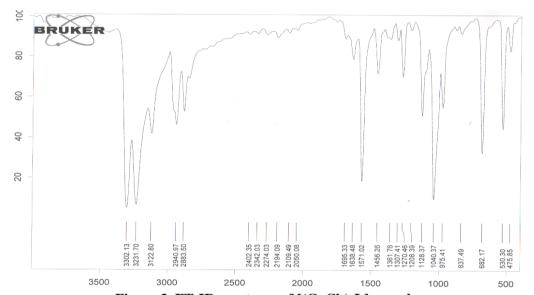
Figure 3. FT-IR spectrum of [(CuCl<sub>2</sub>)<sub>2</sub>L] complex
