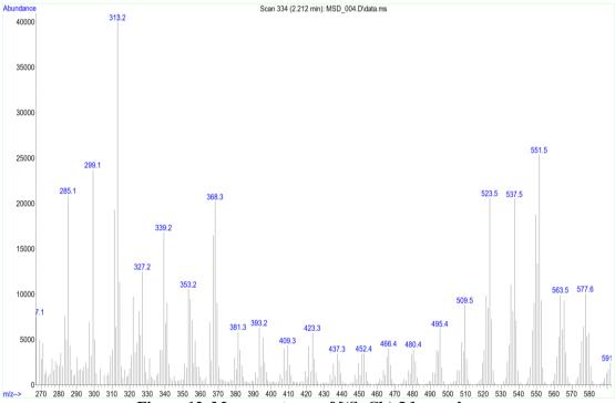
Figure 12. Mass spectrum of [(SnCl<sub>2</sub>)<sub>2</sub>L] complex.
