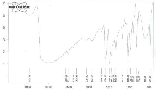
Figure 4. FT-IR spectrum of [(SnCl<sub>2</sub>)<sub>2</sub>L] complex
