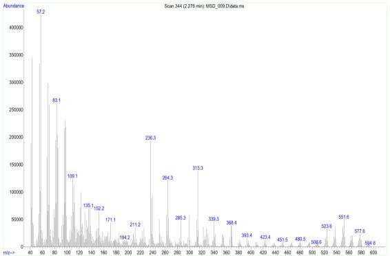
Figure 11. Mass spectrum of [(CuCl<sub>2</sub>)<sub>2</sub>L] complex
