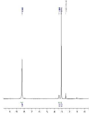
Figure 8. <sup>1</sup>H-MNR spectrum of [(SnCl<sub>2</sub>)<sub>2</sub>L]
