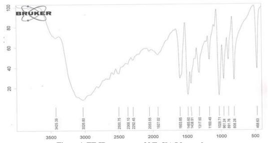
Figure 1. FT-IR spectrum of [(FeCl<sub>2</sub>)<sub>2</sub>L] complex
