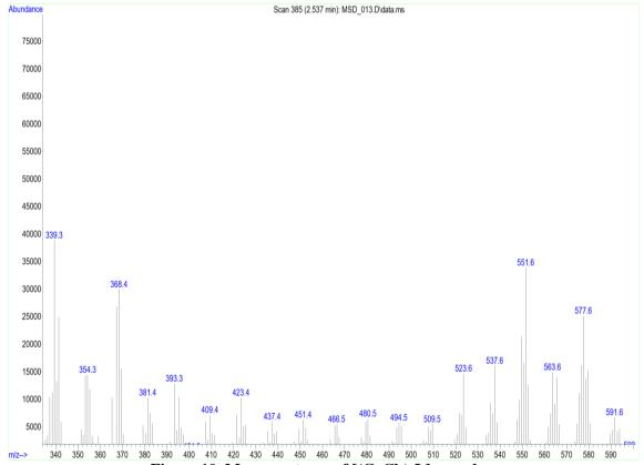
Figure 10. Mass spectrum of [(CoCl<sub>2</sub>)<sub>2</sub>L] complex.
