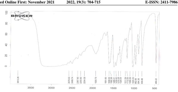
Figure 2. FT-IR spectrum of  $[(CoCl_2)_2L]$  complex
